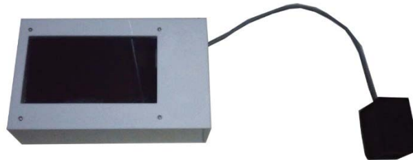
FIGURE 6. Non-invasive blood hemoglobin measurement tool
