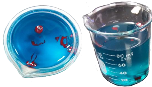
Gambar 6. Penetapan kadar hemoglobin metode cupri sulfat 27
