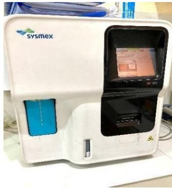
**Gambar 5. Alat Hematology Analyzer Xp-10**
